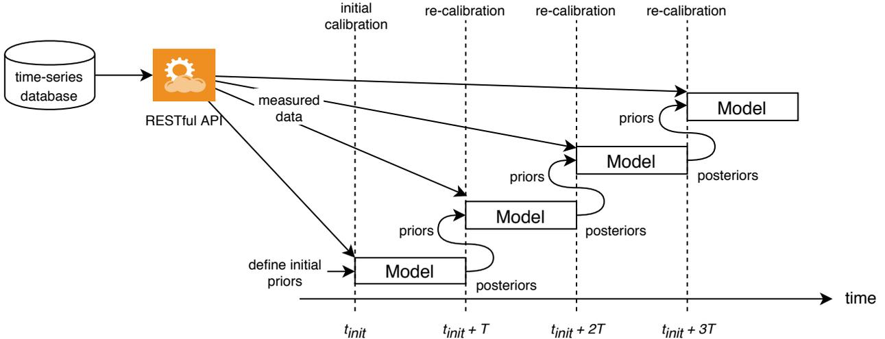
Figure 2: Continuous Bayesian calibration using a sliding time window. The posteriors of the previous calibrated model is used to derive the priors for the Bayesian calibration at the current time-step (Chong et al., 2019)
