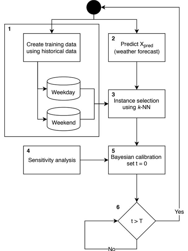
Figure 1: Overview of the proposed framework for the continuous Bayesian calibration of building energy models.
