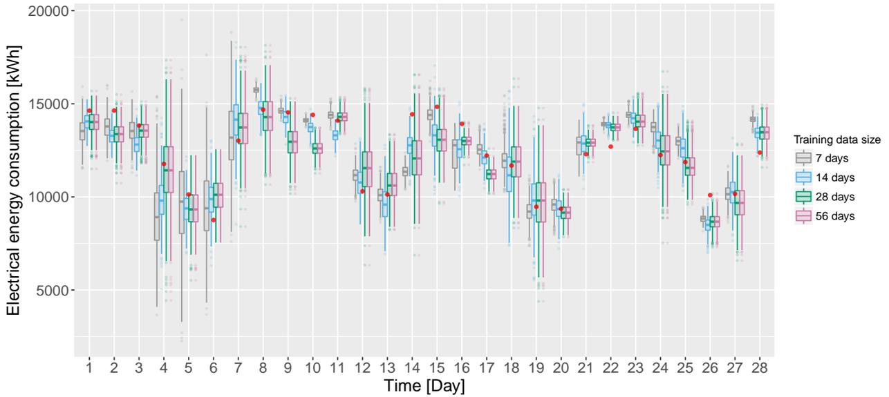
Figure 4: Box and whisker plots showing posterior predictions over test data with different amounts of training data.
