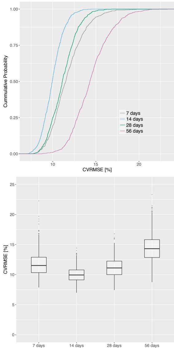
Figure 3: Cumulative distribution (top) and Box and whisker plots (bottom) showing the distribution of CVRMSE computed using samples from the posterior predictions generated by MCMC.
